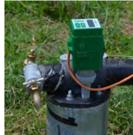
Figure 1. Groundwater level monitoring site with ENO Scientific sensor.
